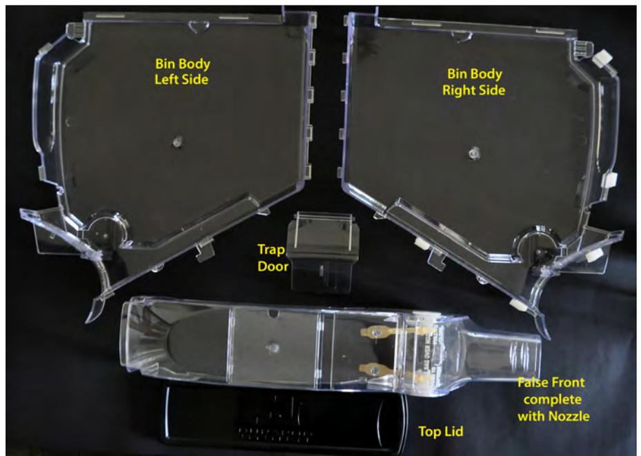
The GD1000 - 4" Bin completely disassembled ready for cleaning
