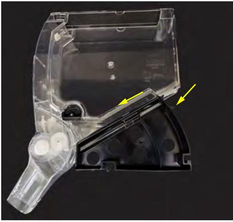
Once complete Bin with Base is removed from shelf separate bin from Base by pushing lever down at rear of base and sliding Bin Body forward to release Body from Base
