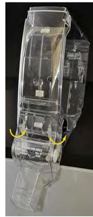
To remove the false front turn the two black clips on the front side of the bin, this spreads the false front for removal.
